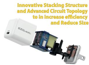
Improved heat dissipation with Heat-Sink
